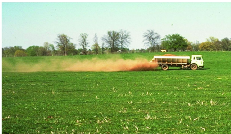
Figure 3. Surface broadcast application of poultry litter to a pasture using a broiler litter spreader truck.
