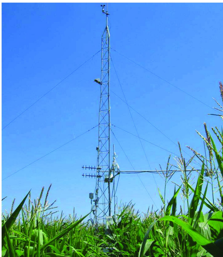
Figure 2. Flux tower for measuring trace gas flux from the plant-soil system.
