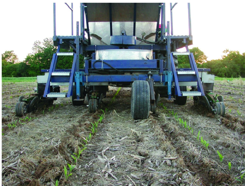
Figure 5. Rear view after subsurface band application of poultry litter using a four-row prototype banding implement.
