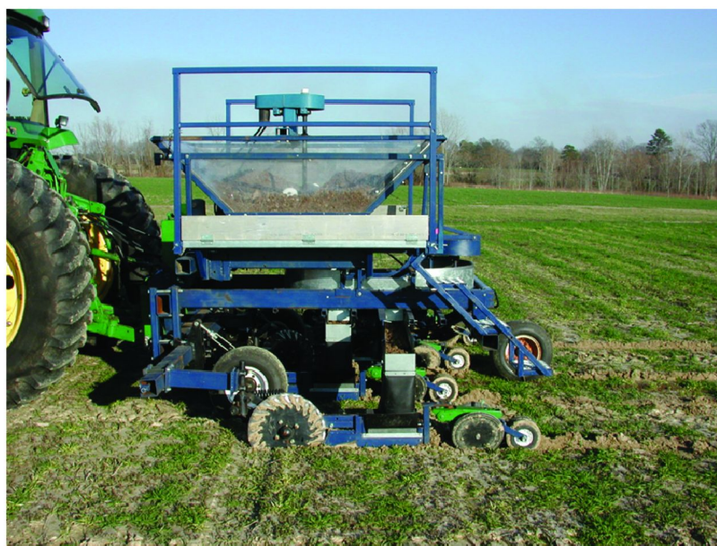
Figure 6. Side view after subsurface band application of poultry litter using the four-row prototype banding implement shown in Figure 5. Direction of forward travel is from right to left.
